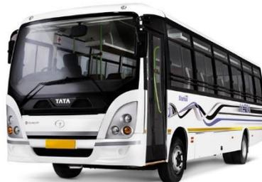
BSIV ready CVs with **Exhaust Gas Recirculation (EGR) and new future leading Selective Catalytic Reduction (SCR)**
